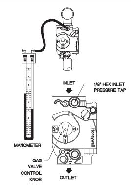
Figure 30 – Measuring Gas Supply Pressure at Combination Gas Valve
